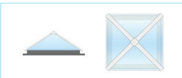
Pyramid unit on builders kerb for 600 - 1500mm span range
